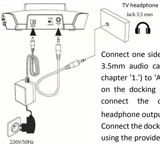
Connect one side of the provided Jack 3.5mm audio cable (see item N°5 in chapter '1.') to 'AUDIO IN' port located on the docking station rear side and connect the other side to the headphone output of the TV.
